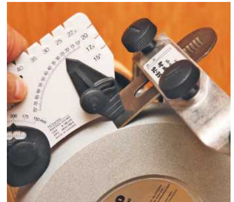
▲ Setting any bevel is consistent and easy with the AngleMaster
